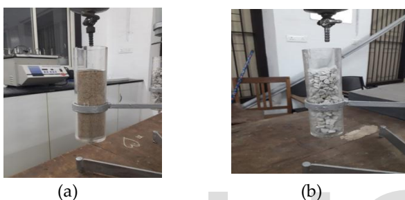
Figure 2: The two different filter media a) sand and b) pumice
