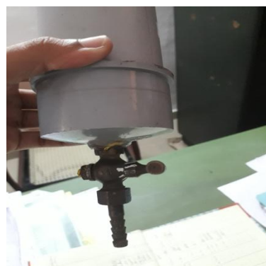
Figure 4: The opening of the outlet valve.
